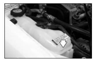
The coolant level should be at the FULL COLD mark. If it isn't, you may have a leak in the radiator hoses, heater hoses, radiator, water pump or somewhere else in the cooling system.
